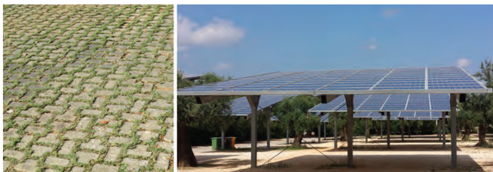
Figure 37: Landscaped surface parking area (left); car parking shading structures that double up as energy-generators (right)
